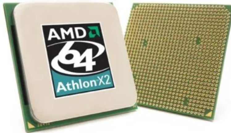
Figure 4. AMD Athlon64 x2 CPU (left is top, right is bottom) with Socket 939
