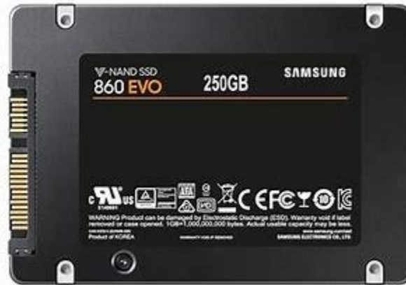
Figure 7. A SATA-interfaced SSD (Solid State Disk) for non-volatile storage.
