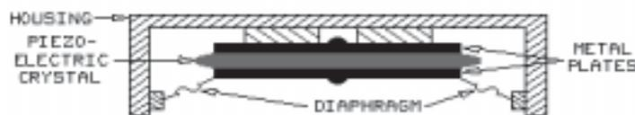
This is a cross-sectional view showing the construction of a piezoelectric transducer. The basic transducer element is a **piezoelectric crystal**, which is usually composed of quartz or a synthetic material.
