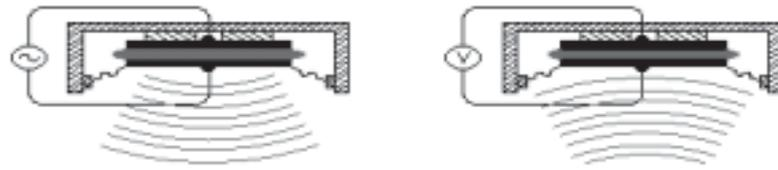
This figure shows that the transducer can be used as either an ultrasonic transmitter or an ultrasonic receiver, depending on how it is configured. The properties of a piezoelectric crystal are such that, when an ac voltage of ultrasonic frequency is applied (right figure), the crystal rapidly expands and contracts.
