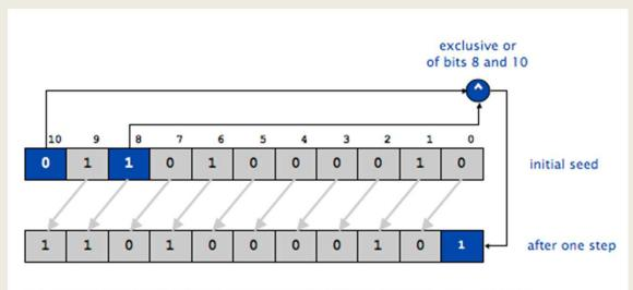
One step of an 11-bit LFSR with initial seed 01101000010 and tap at position 8
