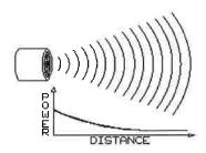
As with any form of radiant energy, transmitted ultrasonic waves grow weaker as they travel farther away from the transmitter.
