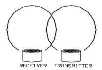
This figure shows the transmitter and receiver as they are positioned on your circuit board, along with their directivity patterns. Because the patterns overlap, the ultrasonic waves from the transmitter are picked up by the receiver, even without a target object. You will see in Exercise 2 how this arrangement limits the measuring range of the tranducers.
