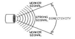
Also, the signal is strongest in the area directly in front of the transmitter. As the angle increases outward, signal strength is attenuated. The angle in which the signal is strongest is called the angle of **directivity**.
