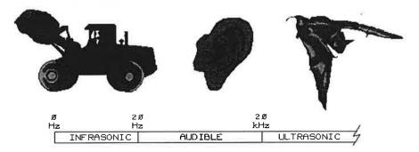
Frequencies above 20 kHz are in the **ultrasonic** range. You cannot hear these frequencies, but they can be detected by instruments and by some animals. Bats, for example, can hear frequencies up to 100 kHz.
