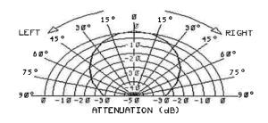
The transducer manufacturer's data sheet often includes a directivity curve, such as the one shown here. At 0° (directly in front of the transducer), signal attenuation is 0 dB. As the angle increases, for example, to 30° left or right of center, attenuation increases to about –7.5 dB.
