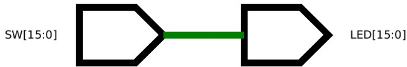
Figure 21. The schematic of a switch checker
